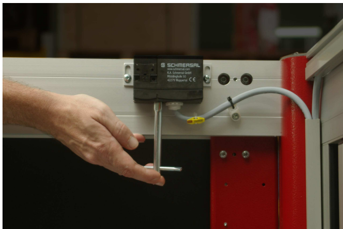
Figure 13: Function conversion door contact
